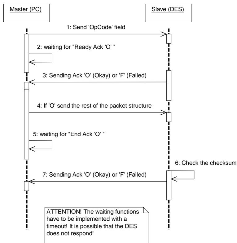
Figure 4.4: Sending a data frame to the DES
