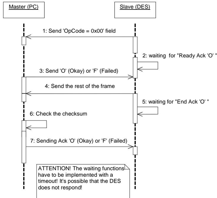
Figure 4.5: Receiving a data frame from the DES
