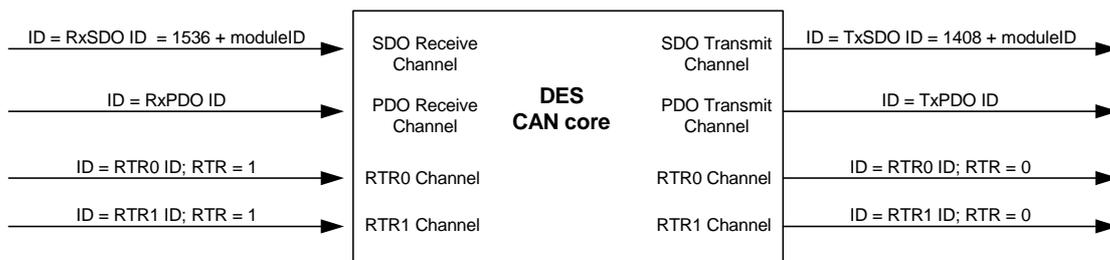
Figure 5.6: CAN communication channels
