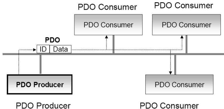
Figure 13: Process Data Object
