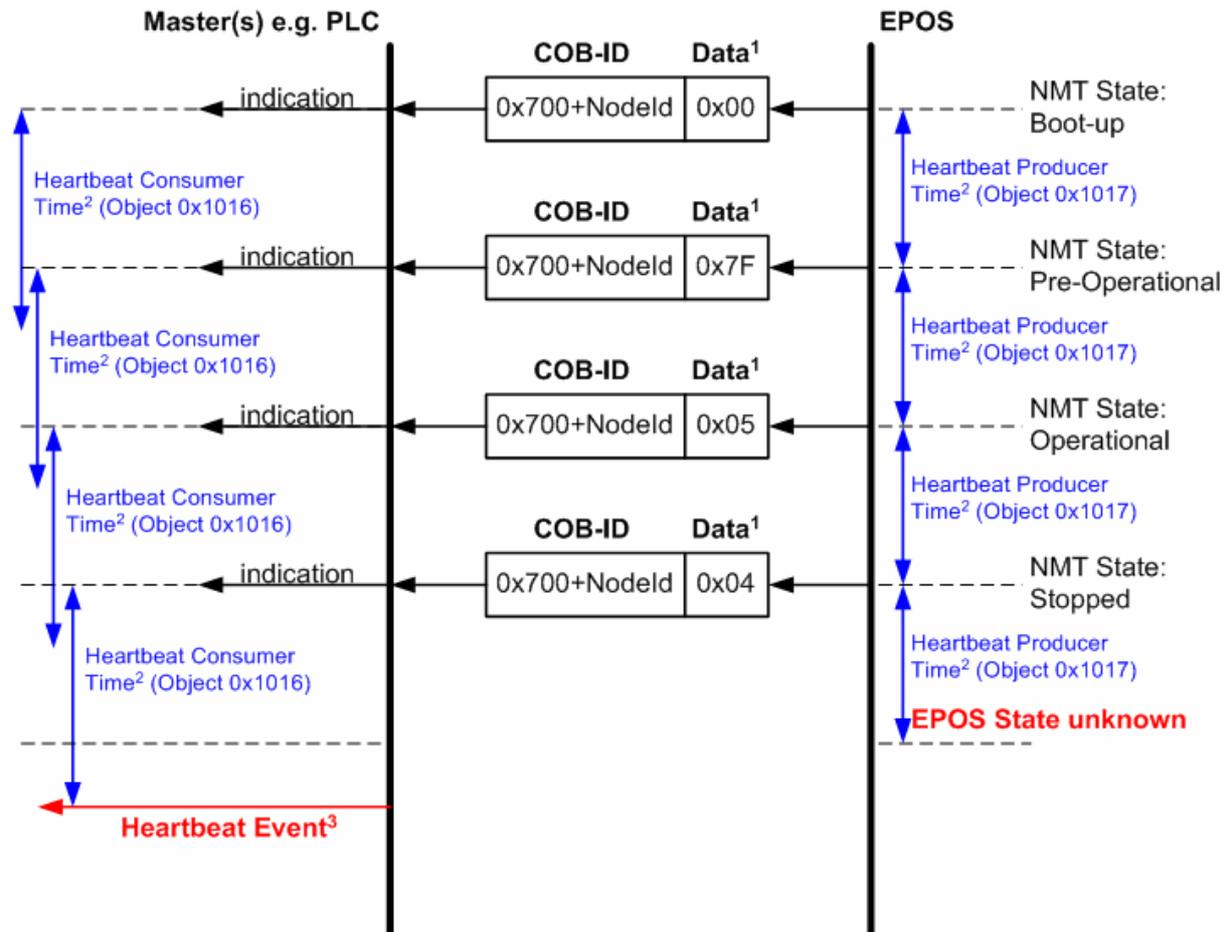
Figure 25: Heartbeat Protocol Timing Diagram
