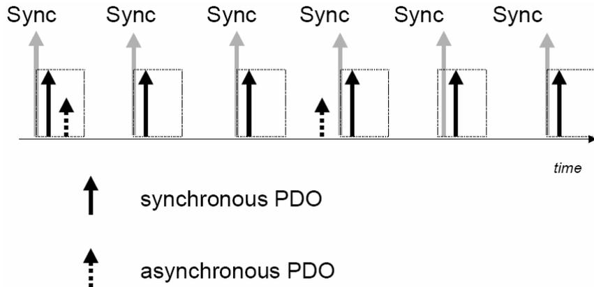
Figure 19: Synchronous PDO
