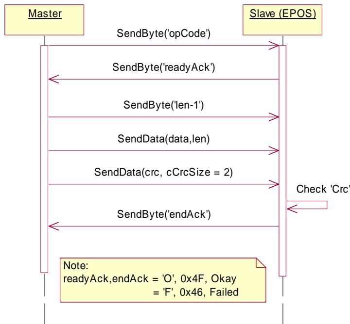
Figure 5: Sending a data frame to the EPOS
