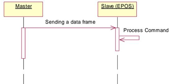
Figure 4: EPOS command without response
