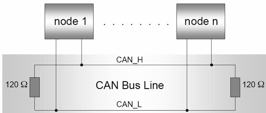
Figure 10: ISO 11898 Basic Network Setup
