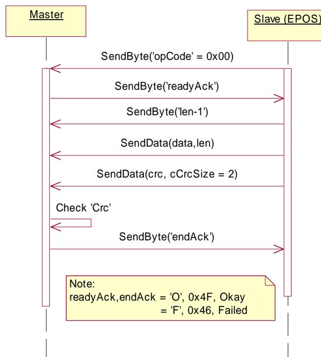
Figure 6: Receiving a response data frame from the EPOS
