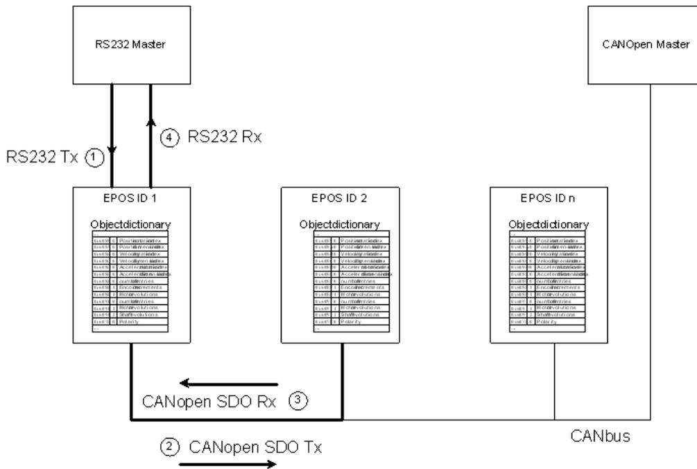
Figure 27: Communication Structure Gateway
