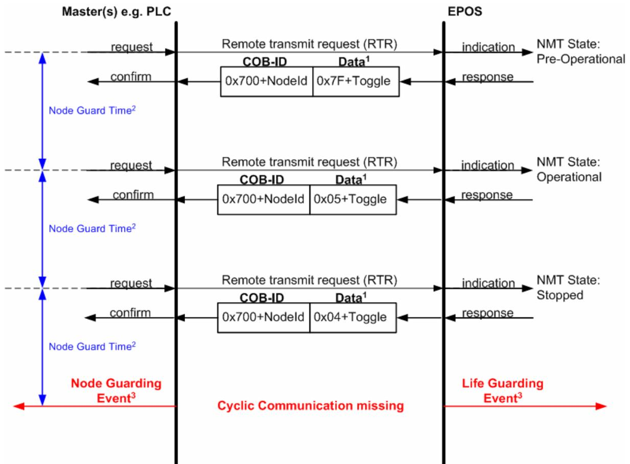
Figure 24: Node Guarding Protocol Timing Diagram
