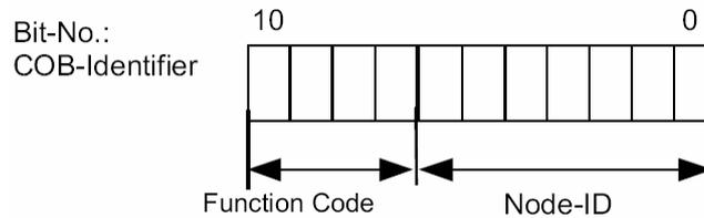
Figure 26: Default Identifier allocation scheme
