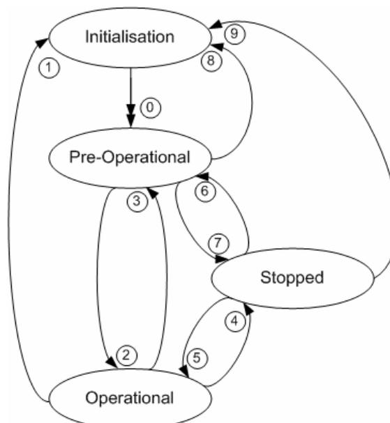
Figure 22: NMT Slave State Diagram
