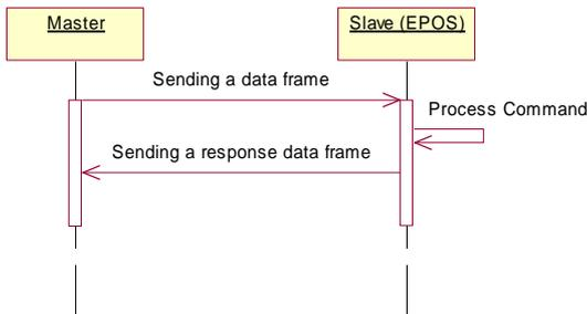
Figure 3: EPOS command with response
